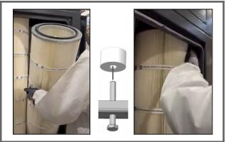
• Screw the fixing screw tight.
