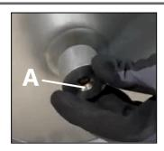
Insert the cartridge holder without a new filter cartridge in one of the cartridge guides.
