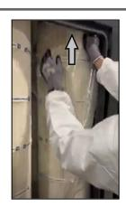
• Unhook the cartridge holder from the cartridge guides.
