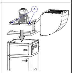
Finally, the components must be joined together by closing the toggle levers. These are supplied loose and must be mounted on site. To do this, it is necessary to screw the toggle levers to the cleaning housing. They are fixed in place using four M6x12 flathead screws.
