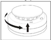
Remove the cover. To do this insert a screwdriver and lift the cover. It is then necessary to pull the black cover off the smokebox.
